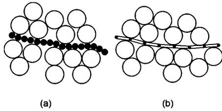
**Fig. 1.** Two different concepts to model soil-inclusion systems with the distinct element method (DEM): (a) full-DEM modeling or (b) DEM–dynamic spar element model modeling. The disks in white represent the soil.
