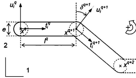
Fig. 4. Geometry and notations
