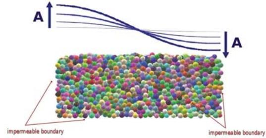
**FIGURE 2.** Representation of the wave action, boundary conditions.
