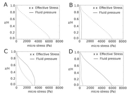
FIGURE 7. Loose seabed - Evolution of the fluid pressure and the effective stress profiles during the simulation.
