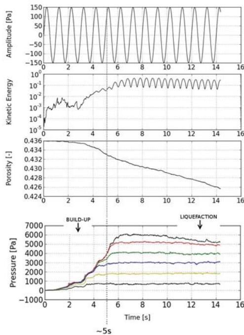
FIGURE 8. Stationary wave - Build-up liquefaction.
