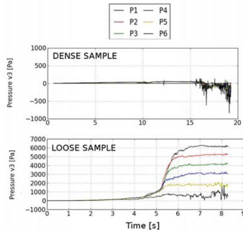
FIGURE 6. Pressure measurements along the symmetric axis of the dense and the loose seabeds (six equally spaced sensors, P1 the lowest, P6 the highest).
