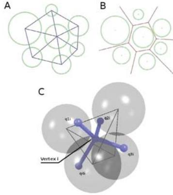
**FIGURE 1.** The PFV geometrical scheme. (A) 2D view of regular triangulation. (B) 2D view of tessellation. (C) 3D view of a pore and its connections.
