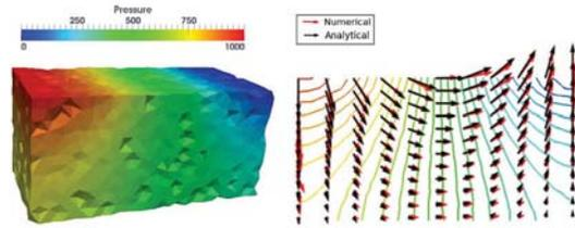
**FIGURE 3.** Wave simulation - (A) Pressure field (half period) with  $A = 500\text{Pa}$  and (B) velocity field and equipotential lines compared with the analytical solution of an equivalent Darcy's problem.
