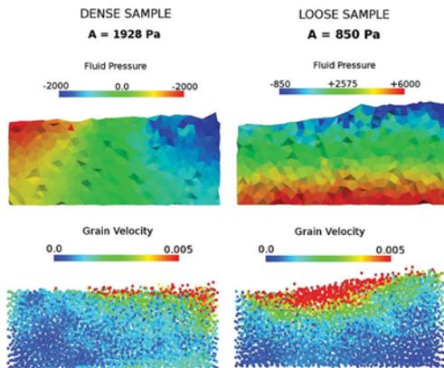
FIGURE 5. Pressure fields and deformation patterns corresponding to a condition of instability for the dense (A) and the loose (B) seabeds.
