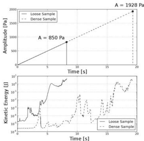
FIGURE 4. Wave action on a dense ( $n = 0.368$ ) and a loose ( $n = 0.436$ ) seabed. Amplitude and kinetic energy evolution.
