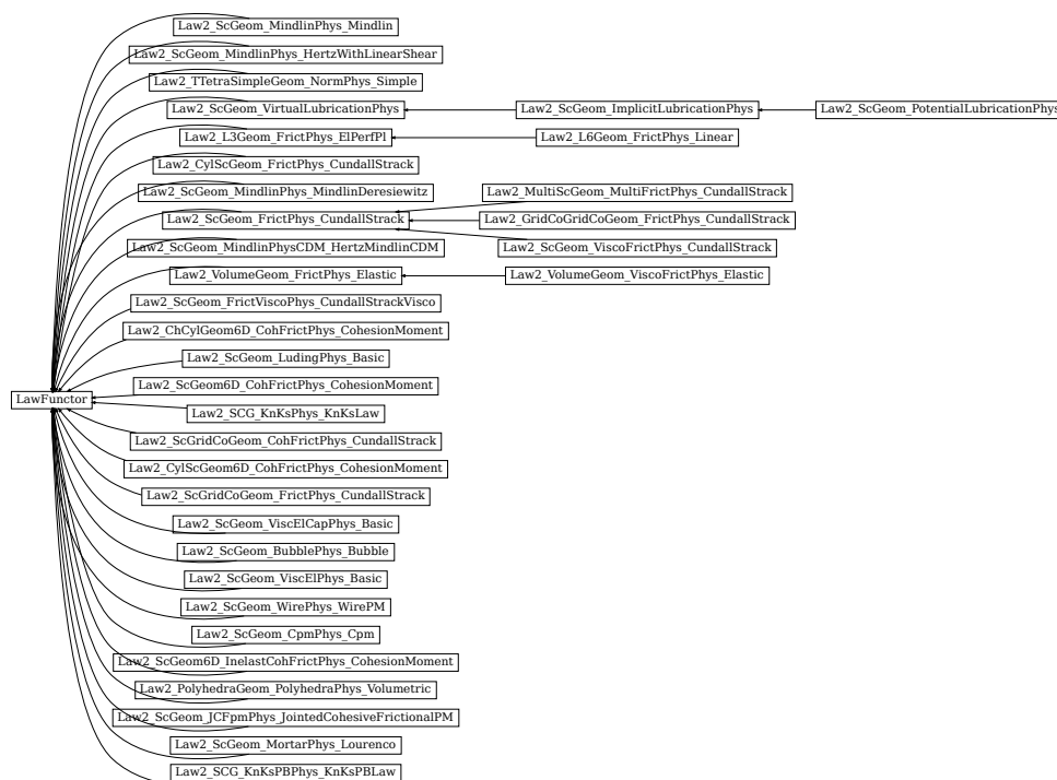
Fig. 36: Inheritance graph of LawFunctor. See also: Law2_ChCylGeom6D_CohFrictPhys_CohesionMoment , Law2_CylScGeom6D_CohFrictPhys_CohesionMoment , Law2_CylScGeom_FrictPhys_CundallStrack , Law2_GridCoGridCoGeom_FrictPhys_CundallStrack , Law2_L3Geom_FrictPhys_ElPerfPl , Law2_L6Geom_FrictPhys_Linear , Law2_MultiScGeom_MultiFrictPhys_CundallStrack , Law2_PolyhedraGeom_PolyhedraPhys_Volumetric , Law2_SCG_KnKsPBPhys_KnKsPBLaw , Law2_SCG_KnKsPhys_KnKsLaw , Law2_ScGeom6D_CohFrictPhys_CohesionMoment , Law2_ScGeom6D_InelastCohFrictPhys_CohesionMoment , Law2_ScGeom_BubblePhys_Bubble , Law2_ScGeom_CpmPhys_Cpm , Law2_ScGeom_FrictPhys_CundallStrack , Law2_ScGeom_FrictViscoPhys_CundallStrackVisco , Law2_ScGeom_ImplicitLubricationPhys , Law2_ScGeom_JCFpmPhys_JointedCohesiveFrictionalPM , Law2_ScGeom_LudingPhys_Basic , Law2_ScGeom_MindlinPhysCDM_HertzMindlinCDM , Law2_ScGeom_MindlinPhys_HertzWithLinearShear , Law2_ScGeom_MindlinPhys_Mindlin , Law2_ScGeom_MindlinPhys_MindlinDeresiewicz , Law2_ScGeom_MortarPhys_Lourenco , Law2_ScGeom_PotentialLubricationPhys , Law2_ScGeom_VirtualLubricationPhys , Law2_ScGeom_ViscElCapPhys_Basic , Law2_ScGeom_ViscElPhys_Basic , Law2_ScGeom_ViscoFrictPhys_CundallStrack , Law2_ScGeom_WirePhys_WirePM , Law2_ScGridCoGeom_CohFrictPhys_CundallStrack , Law2_ScGridCoGeom_FrictPhys_CundallStrack , Law2_TTetraSimpleGeom_NormPhys_Simple , Law2_VolumeGeom_FrictPhys_Elastic , Law2_VolumeGeom_ViscoFrictPhys_Elastic .
